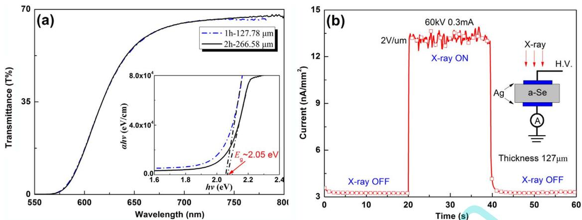
**Fig. 3.** (a) Optical transmittance spectrum and  $\alpha h\nu$  versus  $h\nu$  curves of the as-grown a-Se thick films. (b) X-ray response of the pure a-Se film (127  $\mu\text{m}$  in thickness) with Ag electrodes. The X-ray tube voltage and tube current is 60 kV and 300  $\mu\text{A}$ , respectively.
