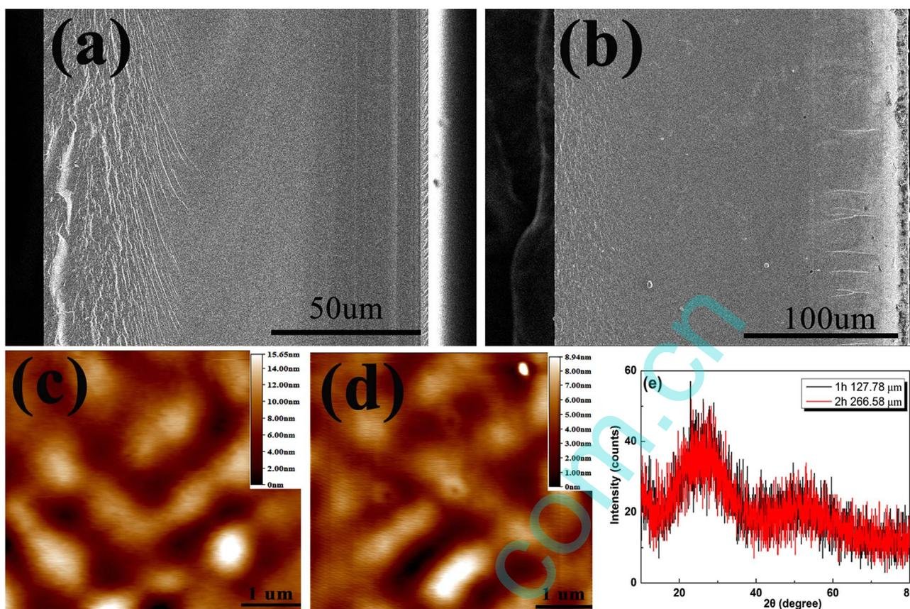
**Fig. 1.** Cross-sectional SEM images of the films deposition for (a) 1 h and (b) 2 h. Surface AFM images of the films deposition for (c) 1 h and (d) 2 h. (e) XRD pattern of the as-grown a-Se thick films.
