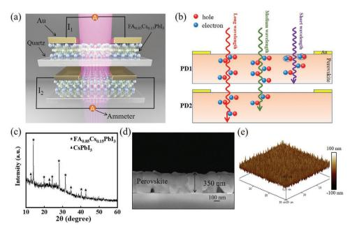
Figure 1. a) Schematic illustration of the as-fabricated wavelength sensor. b) Schematic diagram of the photo-generated carriers for different wavelengths. c) XRD pattern of the as-synthesized  $FA_{0.85}Cs_{0.15}PbI_3$  film. d) Cross-sectional SEM image of the  $FA_{0.85}Cs_{0.15}PbI_3$  film. e) Tapping-mode AFM height profile of the  $FA_{0.85}Cs_{0.15}PbI_3$  film.
