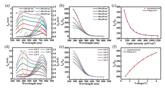
Figure 4. a) The spectral response of both PDs under different light intensities. b) Photocurrent ratio as a function of wavelength, the light intensity changes from 100 to  $500 \,\mu\text{Wcm}^{-2}$ . c) Photocurrent ratio as a function of light intensity. d) The spectral response of both PDs at different voltages. e) Photocurrent ratio as a function of wavelength, the voltage changes from 0.5 to 2.5 V. f) Photocurrent ratios as a function of bias voltage.
