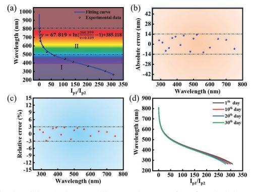
**Figure 5.** a) The dependence of light wavelength on  $I_{\rm pl}/I_{\rm p2}$ , and blue curve is Boltzmann inverse function fit curve. b) Absolute error between the light wavelength of theoretical calculation value and real value. c) Relative error between the light wavelength of theoretical calculation value and real value. d) The variation of the work curve of the photosensor, after storage in air for different times.
