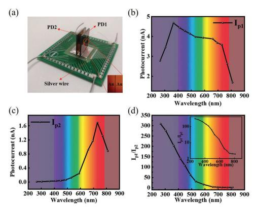
Figure 3. a) A digital photograph of the as-assembled device on PCB. The spectral response of the b) PD1 and c) PD2, the light intensity is 300  $\mu$ Wcm<sup>-2</sup>. d) The  $I_{p1}/I_{p2}$  under different light wavelengths, the inset is the photocurrent ratio  $(I_{p1}/I_{p2})$  in logarithmic coordinates.
